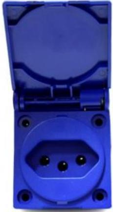
Sockets with (4 mm) diameter must be used, for devices with a rated current of up to 10 amps, and (4.8 mm) plugs for equipment that operate with more than 10 Ampere in up to 20 amps. This difference was necessary to ensure safety, since it prevents the connection of higher power equipment at a point that was not specifically designed for this action.
